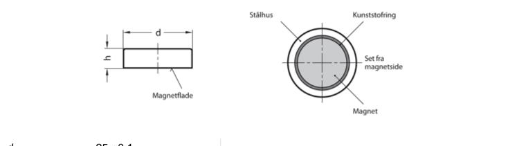
d =  $25 \pm 0,1$ h =  $7 \pm 0,3/-0,1$ Holding force N = 40Material = HF hard ferrite -  $200^{\circ}$  C
